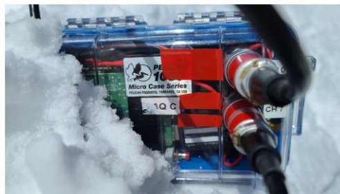
Figure 3 – Raspberry Pi-based data acquisition systems used to collect high-speed pressure data from Larcor microphones.
