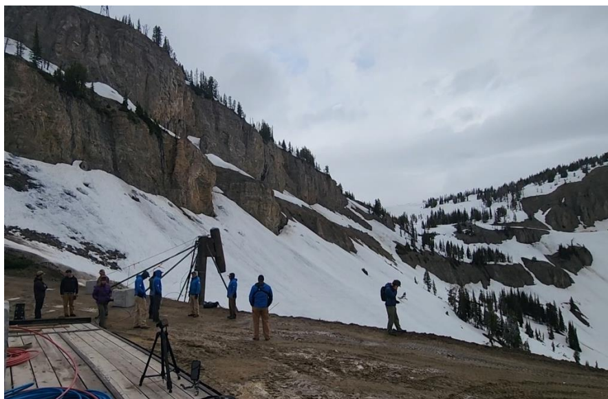
Figure 1 – Prototype BW Exploder RAC System designed by Eric Bressler of Alpine Infrastructure installed at Jackson Hole Mountain Resort for system testing.
