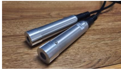
Figure 2 – 10 psi Larcor microphones used to measure explosive blast wave air pressures.
